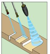
Legacy's Revolution is the best of both worlds: deep cleaning impact of a 0° nozzle with the fast cleaning of a widecoverage fan spray nozzle.
