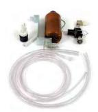
Magnetically activated "snap acting" float valves provide full water flow to activate the chemical proportioners. There are two basic sizes to give a choice of water flows as shown in the table below. Chemical feed rate is adjusted by metering screw or threaded metering tips. The compact 440 float valve is made of Celcon® plastic and is easily accessible for field maintenance.
